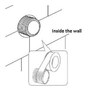
3. Continue screwing the thread into the fitting until a seal is created and the outlet for the hose is pointing downwards and, the wall elbow is flush with the finished wall. Silicone can be applied if necessary.
