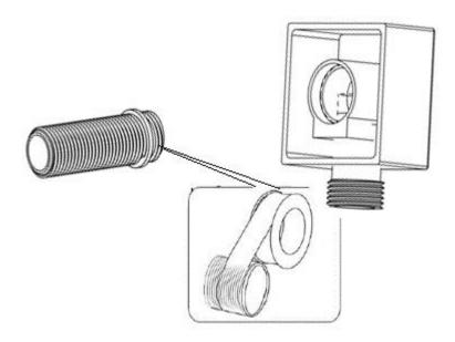
2. Apply sufficient PTFE to the thread of the long thread of the wall elbow which will go into the wall. Place the thread through the hole in the wall and screw this into the fitting within the wall.
