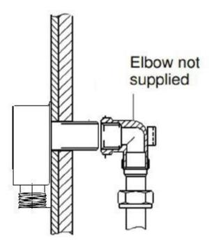
**Please note:** Once installation is completed, turn on the water supply and check for any leaks
